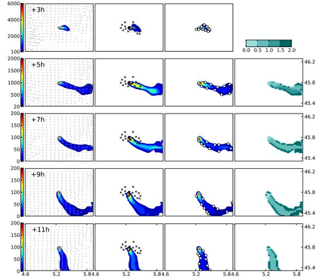
First column: reference simulation (truth) knowing the true source. Second column: forecast of plume using data assimilation of fixed observations. Third column: forecast of plume using data assimilation of fixed and adaptive observations. Fourth column: contrast factor between the second and third column.
