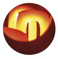
which slowly fatten into "rods" of 99.9999% pure (or better) polysilicon. When pre-heated to around 1100°C, the silicon filaments/rods growing beneath the reactor cover can catch about 20% of the silicon atoms that pass through the reactor in
