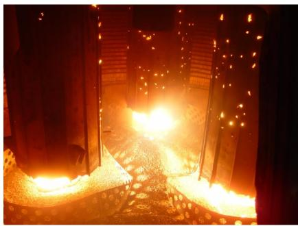
Figure 2. In the silicon smelter, three 1-meter diameter carbon electrodes penetrate the surface of the charge of coal, coke, woodchips, and quartz rock. Each electrode is 10-20 meters tall.
