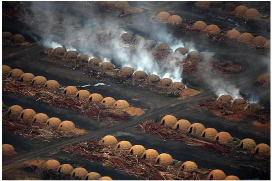
By weight, up to  $\sim 90\%$  of the wood harvested is lost to the atmosphere as CO, CO<sub>2</sub>, smoke, and heat, so as much as ten tons of raw wood must be burned to produce a single ton of wood charcoal. [28][33] A few silicon producers claim to use dedicated "charcoal plantations," but such plantations are limited in scope, so they can only supply a fraction of the overall demand for carbon in silicon production. [29-31]
