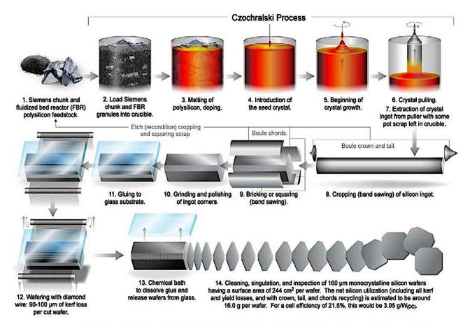
Process flow for making monocrystalline-silicon wafers via Cz crystal growth
